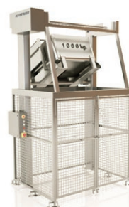
Lifting and Tipping Machine Tilting Height: max. 6000mm KR-2431210
