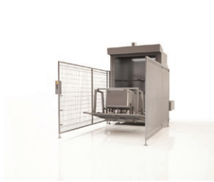
Eurobin Washing Machine inc Safety Light Barrier KR-2232104
